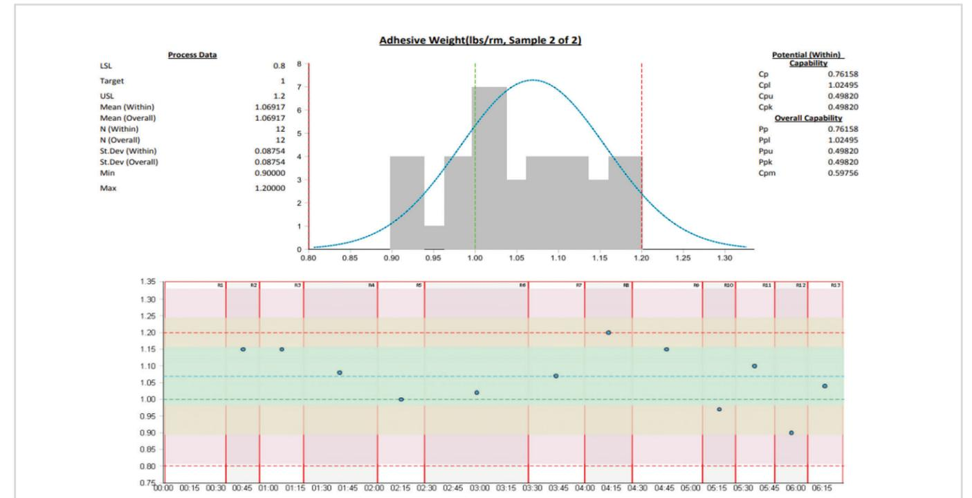
In the screenshot above, the ei<sup>3</sup> system summarizes measurements taken in the continuous manufacturing process, visualizing the spread of the measurement variable across the desired value. Cut-off lines on either side visualize allowable bands. Operators immediately see if the plant is operating at excess waste, i.e., measurements falling outside those bands.
